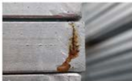
Overgrinding leading to poor penetration and chemical weep
