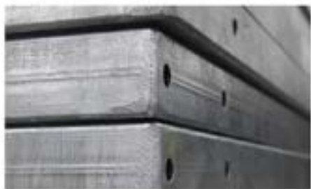
Coarse grinding leading to rough finish
