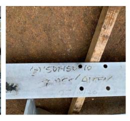
The photos illustrate typical paint markings on material which have to be either ground off manually or wiped down with strong paint removers to eliminate the paint prior to acid pickling. This is extremely time consuming but failure to remove this paint can result in uncoated areas after processing that will fail the BS 1461 standard, as shown in the photo on the right above. These items will then require re-galvanizing at extra cost. This will also delay the turnaround on your order.
