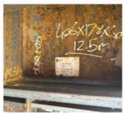
The photos above illustrate various material with labels on them. The label has to be removed prior to galvanizing. This is usually carried out by being mechanically ground off or chemically wiped down. This will then allow our acid pickling to clean your material and for the zinc to react to form the galvanized coating. Our chemical pre-treatment processes won't remove the label and glue residue meaning unfortunately the extra work carried out is chargeable due to the additional time taken.
