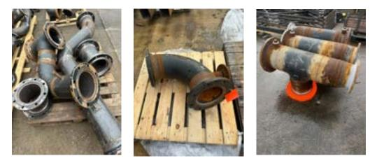
The solution is always have pipework shotblasted. This can be made even easier by carrying this out prior to fabrication making it less complicated for the shotblaster.
