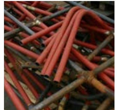
Illustrated above are several common types of material with paint on them. The paint has to be removed prior to galvanizing by either shotblasting, being ground off or chemically wiped down. This will then allow our acid pickling to clean your material and for the zinc to react to form the galvanized coating. **Unfortunately this extra work is chargeable due to the time involved removing the paint as our process doesn't remove it.**
