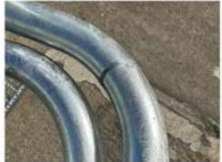
These marks are common feature of Hot Dip Galvanizing and are not detrimental to the overall protection of the material, however if required, can be repaired using a good quality zinc rich paint as recommended by BS EN ISO 1461 - 2022 - article 6.3 Renovation.
