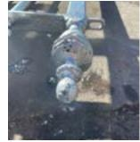
If any problems are experienced with the hot dip galvanizing of castings, they can usually be traced back to the surface condition of the castings. Imperfections can include burnt-on moulding sand, oxides from the annealing process, traces of graphite, or pollution or surface flaws such as shrinkage holes.
